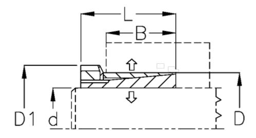
$\begin{array}{lll} \text{B mm} & = 18 \\ \text{D1 mm} & = 38 \\ \text{d H8 mm} & = 19 \\ \text{D mm} & = 30 \\ \text{Fit tolerance} & = \text{Aksel h8, Nav H8} \\ \text{F kN torque} & = 20 \\ \text{L mm} & = 31 \\ \text{P N/mm2 surface pressure on shaft/hub} = 90 \end{array}$
